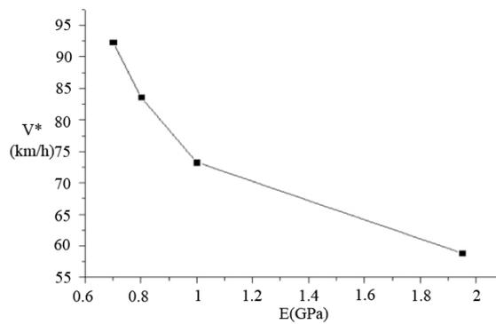
Fig. 5. Critical (minimal) vehicle velocity leading to initiation of fracture in asphalt as a function of asphalt elastic modulus.
