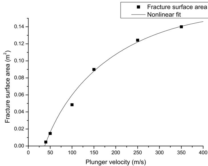
**Figure 2.** Fracture surface area—plunger initial velocity dependence.
