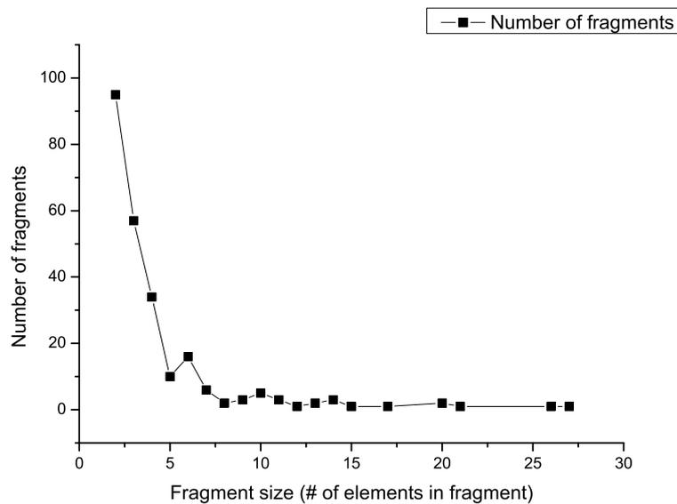
**Figure 5.** Number of fragments of each size for the plunger velocity 250 m/s and 1  $\mu\text{s}$  incubation time value.
