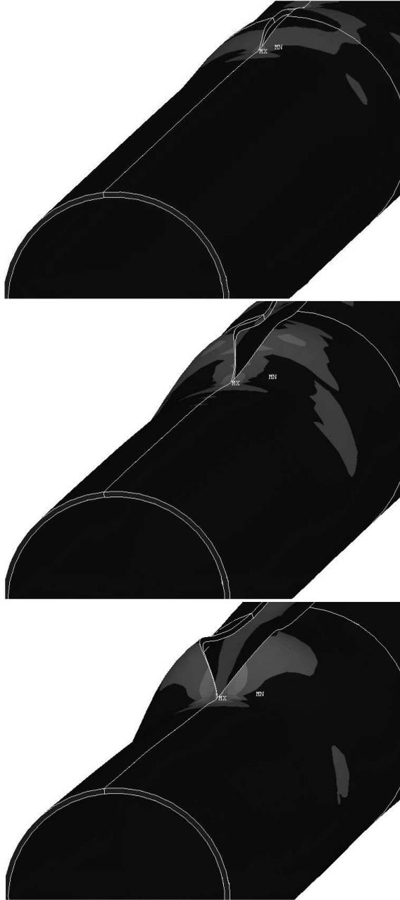
Figure 5: Pipeline with a macroscopic crack
